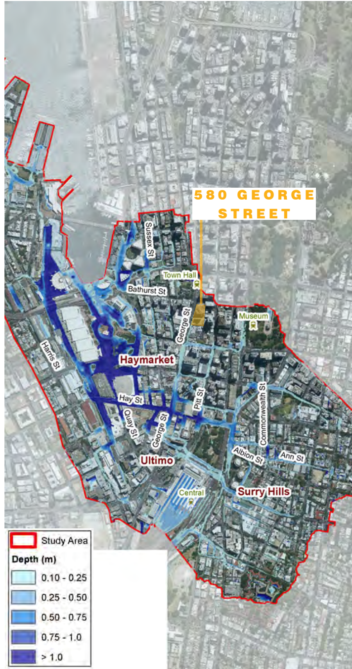
PEAK FLOOD DEPTH PMF DESIGN FLOOD EVENT
